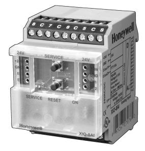
The XIO-8AI Analog Input Module has 8 inputs, which can be wired to passive resistance sensors or active sensors (voltage inputs) as needed. For active sensors, the permissible input D.C. voltage is 0 to 10 V. Resistance sensors can work in a range of 40 Ohm to 4 Megohm. The setting of the ranges and input of the sensor characteristic curves with 10 support points for linearization is performed with an LNS<sup>®</sup> plug-in.
