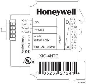
Fig. 6. XIO-4NTC Pin Assignment.
