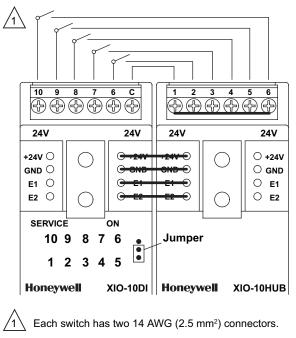
NOTE: ADDITIONAL WIRING POINTS, ONLY ONE WIRE / CONNECTOR; ALSO FOR RELAY OUTPUT.
