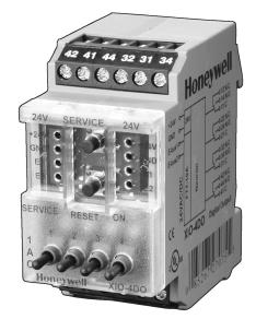
The XIO-4DO Digital Output Module is used to switch electrical units, such as fans, pumps, etc. Four independent relays with one potential-free change-over contact are available for this purpose.
