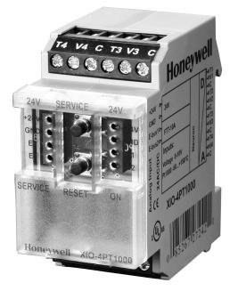
The XIO-4PT1000 LON Analog Input Module is a LON module with 8 analog inputs, 4 temperature and 4 voltage, suitable to collect temperatures with PT 1000 sensors and voltages. In a LON installation, all 8 inputs can be scanned simultaneously by standard network variables, SNVT.
