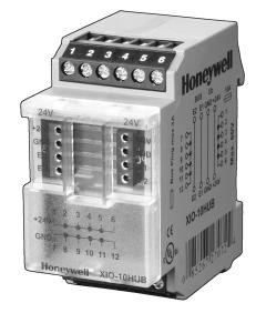
The XIO-10HUB Terminal Module provides additional support terminals, e.g., for the power supply of external drives. The terminals are not connected to the internal 24 V and ground wires; thus, they can be used individually. Six (6) terminals each are bridged among each other.
